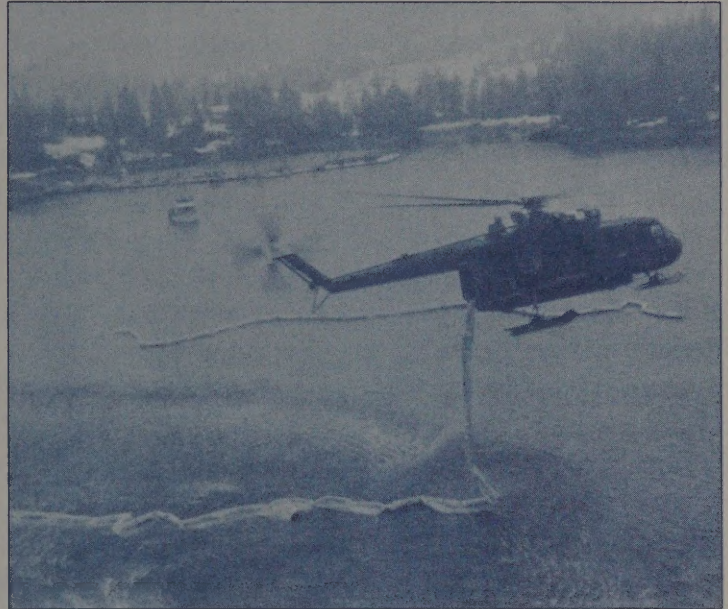
Helicopter deploys an oil boom to protect a fish hatchery in Prince William Sound. Photo by Irene Collie, AK Civil Air Patrol.
